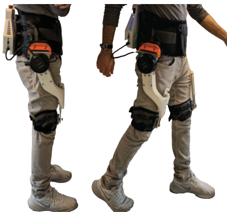
Fig. 6: The active hip orthosis eWalk.
