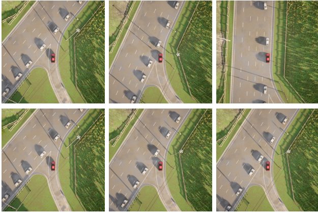
Fig. 3. Qualitative example of proactive merging with closed-loop planning. The top row is from our proposed closed-loop planner and the bottom row is from the open-loop variant of our planner. Frames are in sequential order from left to right. The closed-loop planner merges proactively in front of other cars, causing the car behind to yield to the ego-agent. The open-loop planner does not predict that the ego will affect the behavior of other cars, so it does not attempt to merge.
