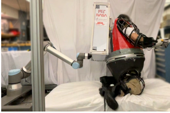
Fig. 8. Test subject wearing the SuperEMU performing a kneeling to upright transition with the assistance from SuperLimbs.
