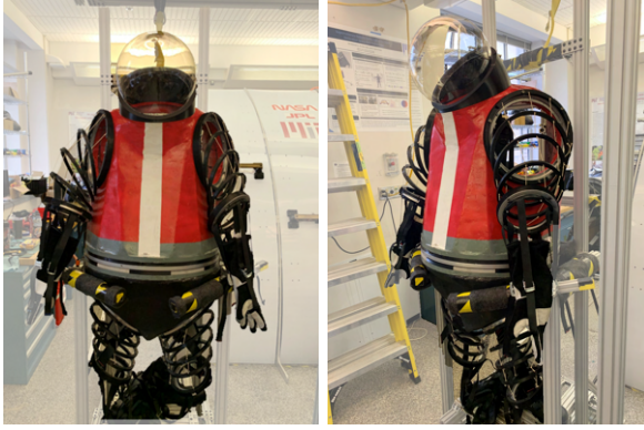
Fig. 3. Supernumerary Robotic Limbs Extra-Vehicular Mobility Unit testing prototype (SuperEMU).
