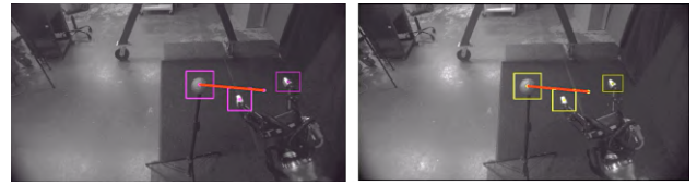
Fig. 11: Left : Left error vector (red) in left camera image calculated between features tracked in the magenta boxes, Right : Right error vector (red) shown in right camera image calculated between features tracked in the yellow boxes
