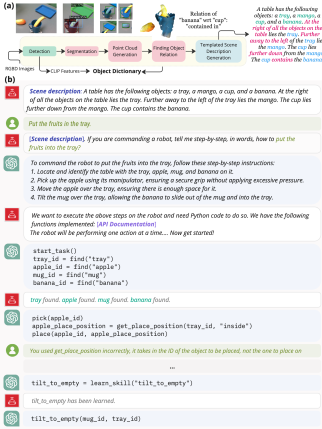
Fig. 2: (a) From RGB-D images, our perception module obtains information about the objects and their relations, creates an object information dictionary, and generates a scene description (detection, object pairs corresponding to given object relations, and the template is in black). (b) An example showing the interaction between the robot, the user, and the planner.
