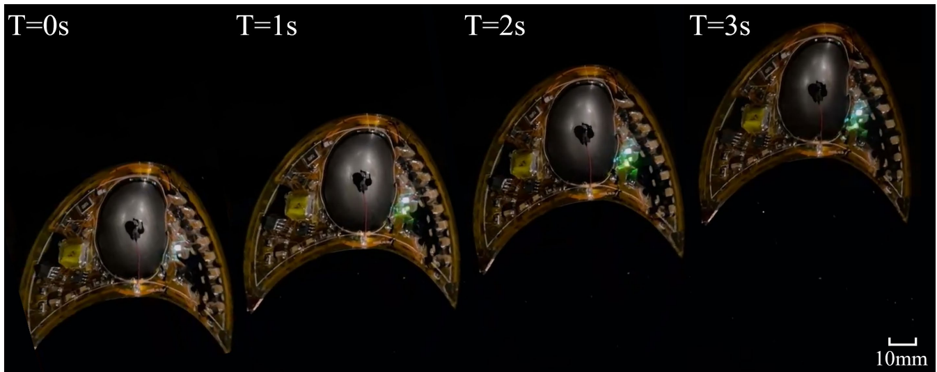
Figure 6. The variation of swimming distance of robotic fish over time. The untethered robotic fish has a downstream speed of 17.0mm/s at a fin flapping frequency of 10hz.
