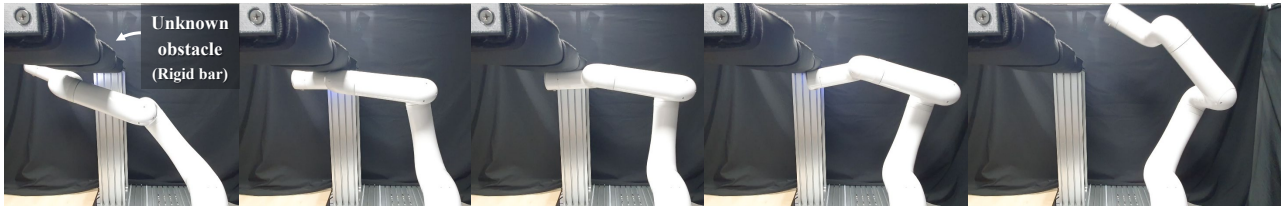
Fig. 4. Snapshot for the experiment 1. The robot complies with the unknown obstacle obstructing the trajectory.
