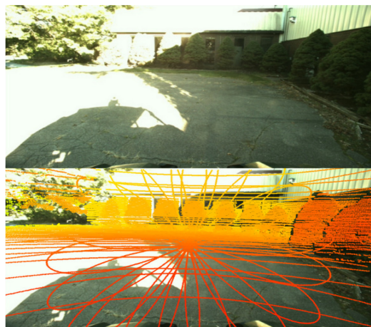
Fig. 10: An example of the overlap between a single scan from all 3 LiDARS and our camera. Points are colored by forward distance from the vehicle.
