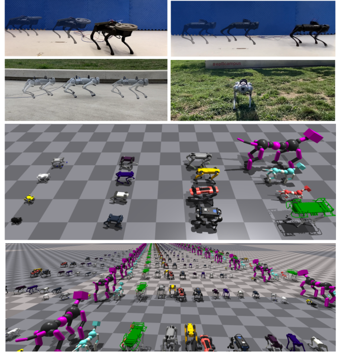
Fig. 1: Simulation and experiment snapshots of training and deploying a single policy to control 16 different robots. Videos: https://miladshafiee.github.io/ManyQuadrupeds/
