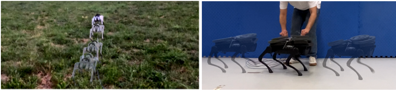
Fig. 5: Left: Snapshots of Go1 trotting on uneven grass. Right: Snapshots of A1 carrying 10 to 15 kg. The robot starts trotting with a 10 kg mass, and then an additional 5 kg is added. The robot successfully walks despite never having encountered any such disturbances during training.
