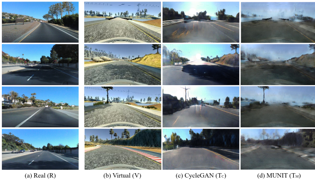
Fig. 3: Sample images of various datasets. (a) the Nvidia dataset [7] (real dataset, denoted by R ). (b) the Udacity dataset [1] (virtual dataset, denoted by V ). (c) style-transferred images from virtual to real using CycleGAN [47] (denoted by T_C ). (d) style-transferred images from virtual to real using MUNIT [21] (denoted by T_M ). All datasets to be released.
