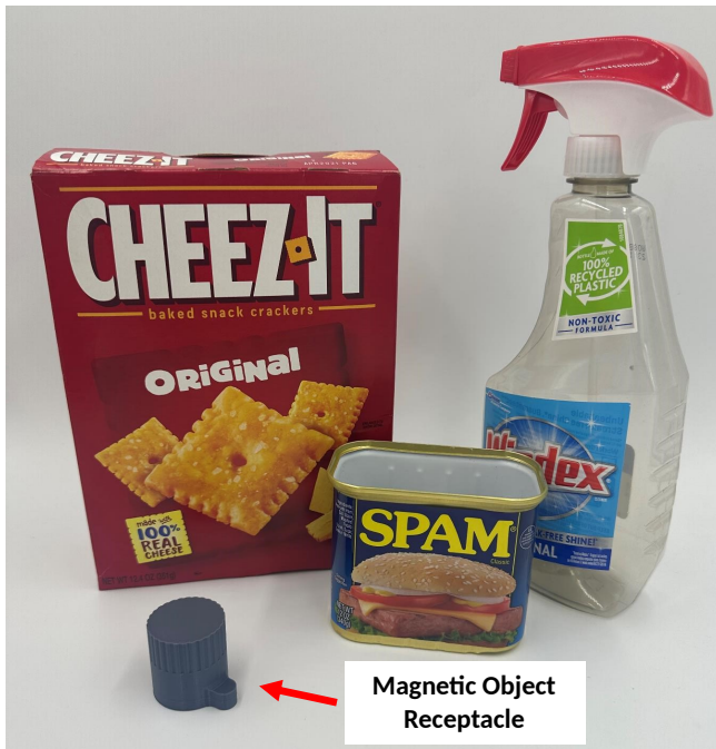
Fig. 5. The magnetic object receptacle is pictured in the bottom left, with three objects from the YCB data set [13] — a CheezIt box, SPAM can, and spray bottle. Using these objects with the GRM is straightforward, simply a hole must be cut in the bottom and the receptacle glued in.
