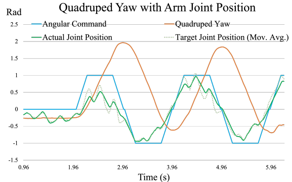
(a) Simulation results with robot running at 1m/s . The desired (dotted green) and actual (solid green) first arm joint positions are shown with the quadruped base angular velocity command (blue) and yaw (orange).
