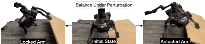
Fig. 5: Robot stabilization under external perturbations. The robot with a locked arm fails to maintain balance. For actuated arm, instead of moving the arm to its left for changing the CoM, as shown in section VIII, the arm relies on the dynamic torques to mitigate the impulse perturbation, resulting the arm moving to its right.
