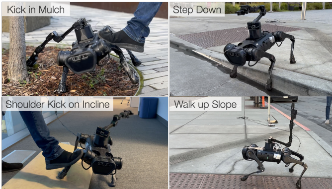
Fig. 4: Physical Experiments under different scenarios. Our system, only trained on fractal terrains with external pushes, is successfully deployed on different real-world scenarios. The arm is at different configurations under different scenarios.
