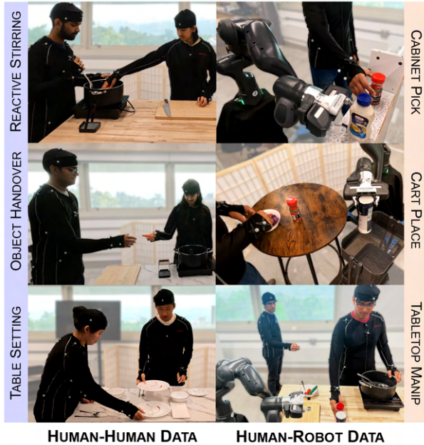
Fig. 3: Collaborative Manipulation Dataset (CoMaD) consists of Human-Human and Human-Robot interaction data. We collect data on three different H-H tasks and three different H-R tasks across several subjects. The bottom right image shows our tele-operation setup for paired human-robot data collection.
