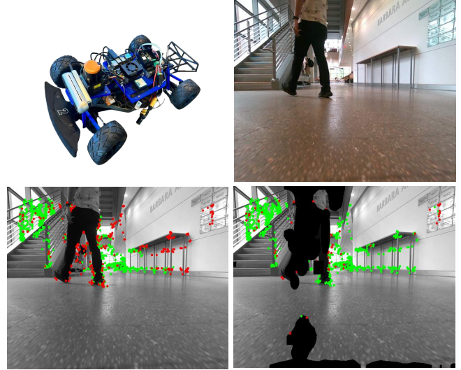
Fig. 6: Experiment Setup(Top Left), Raw Image(Top Right) with dynamic objects inducing outliers using an orthogonal range of movements. Inliers vs Outliers distribution on raw image space vs L-DYNO (Bottom Right).
