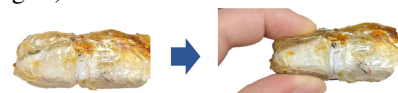
Fig. 2. Soft rubber skin. The surface is deformed when pressed with a human finger.
