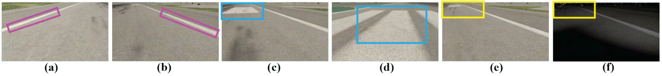
Fig. 4: Failures detected by AD. (a, b) Images correspond to the aircraft being close to the runway boundaries (highlighted with the magenta bounding boxes). (c, d) The visual controller confuses the runway markings (highlighted with the cyan bounding boxes) with the centerline and ultimately leads to a system failure. (e, f) Image (f) is (accurately) not classified as an anomaly during the night time (the same image is classified as anomaly during the day, shown in (e)), as the runway lights (highlighted with the yellow bounding boxes) help the visual controller to predict its position accurately and thereby avoid failure.
