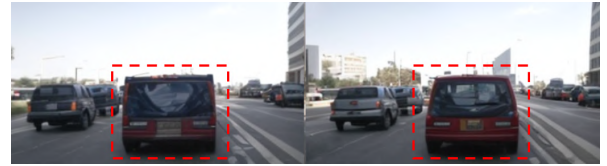
Fig. 3. The impact of shape refinement on the final image generation is evident. Without refinement, the resulting image (left) resembles a cube. In contrast, the refined version (right) exhibits a more natural form.
