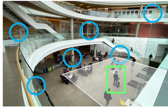
Fig. 3: Hardware setup for the TBD Pedestrian Dataset. Blue circles indicate positions of RGB cameras. Green box shows our suitcase robot pushed through the scene. The white area is where trajectory labels are collected.
