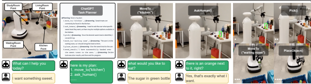
Fig. 8. Showcase of the interactive visual grounding in robotic manipulation tasks on the mobile platform.
