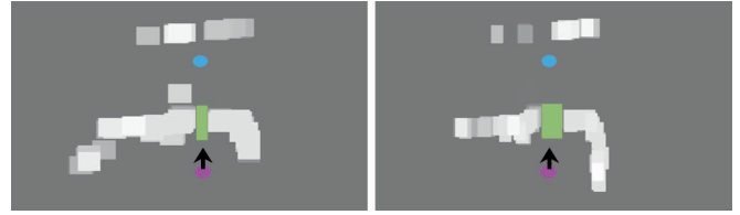
Fig. 3: The robot's position and its goal are denoted by the pink and blue circles respectively. The robot's heading and goal direction coincide in this case. [Left]: Uniformly inflating obstacles using an e \times e kernel with all ones near a narrow passage closing up the available free space (green rectangle). [Right]: Adaptively inflating the obstacles based on the robot's goal direction preserves the free space while inflating the obstacles in the direction opposite to the robot's goal direction.
