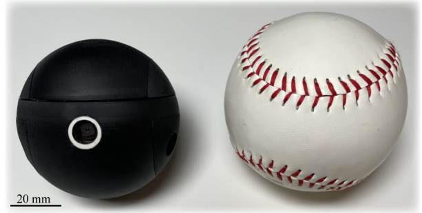
Fig. 1. The assembled robot (64 mm) beside a baseball (73 mm) for scale.
