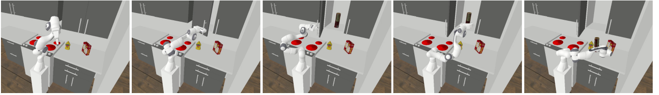
Fig. 5. Snapshots of the trajectory planned using CVQ-MPT for the Panda Arm completing the multi-sequence task (from left to right). CVQ-MPT can plan trajectories for various types of planning constraints in complex environments.
