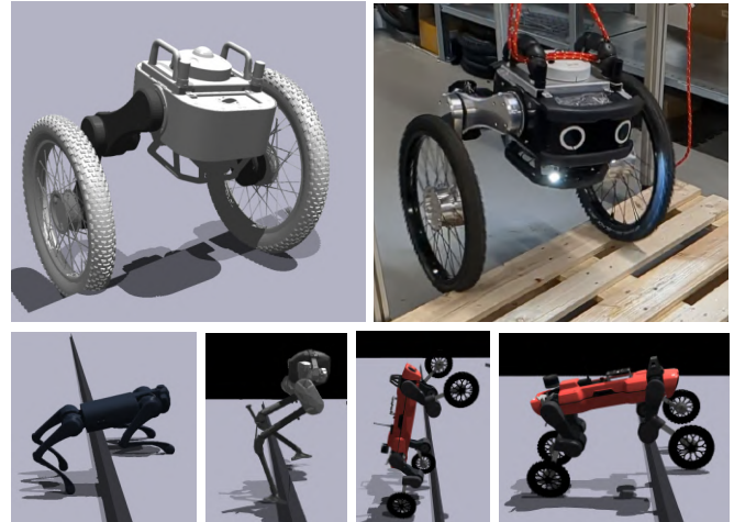
Fig. 1: Proposed Method: Ascento Robot, Unitree Go1, Cassie and ANYmal on Wheels climbing steps.
