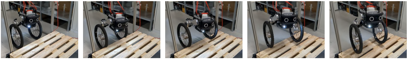
Fig. 6: Real World Results: The Ascento robot going up a 15cm step with our learned policy. Images are taken at 4 Hz.
