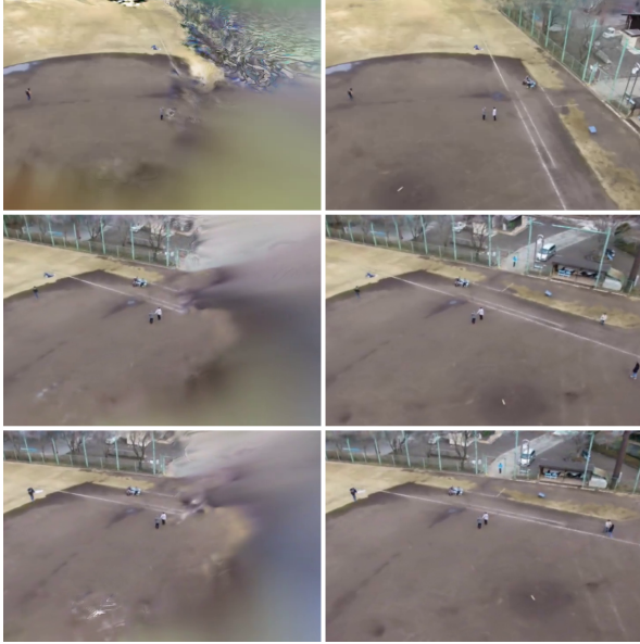
Fig. 5. Left images show novel views from a validation set rendered by the stock K-Planes algorithm trained on a subset of the Okutama-Action dataset. Right images show novel views from the same validation set but rendered with our extended K-Planes algorithm trained on the same subset of data and same hyperparameters.
