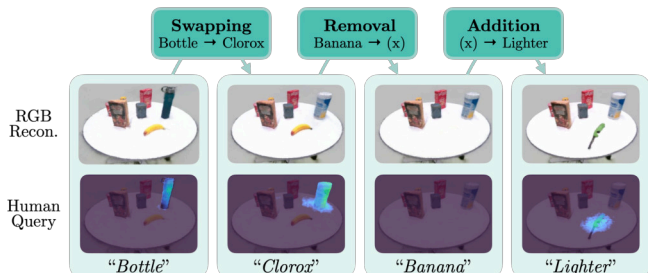
Fig. 5: Sequential scene update. Scene reconstructions are shown in the middle, and human queries are shown at the bottom. As the scene updates, the heatmap for human queries updates accordingly.
