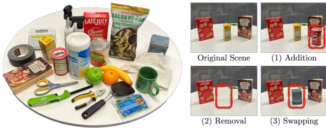
Fig. 4: Experiment setup (Left): Test objects; (Right): Three types of scene changes included in evaluation. Red box denotes the changed scene region.
