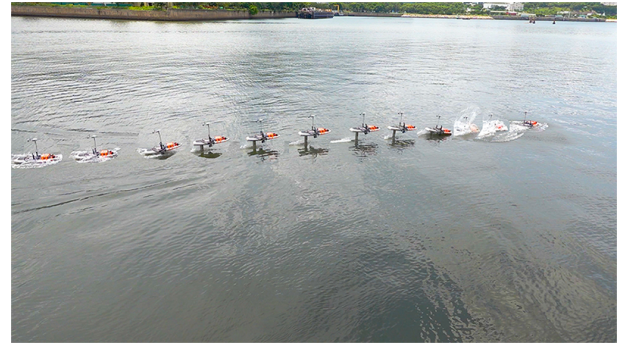
Fig. 7: Test results of Sea-U-Foil in foilborne mode
