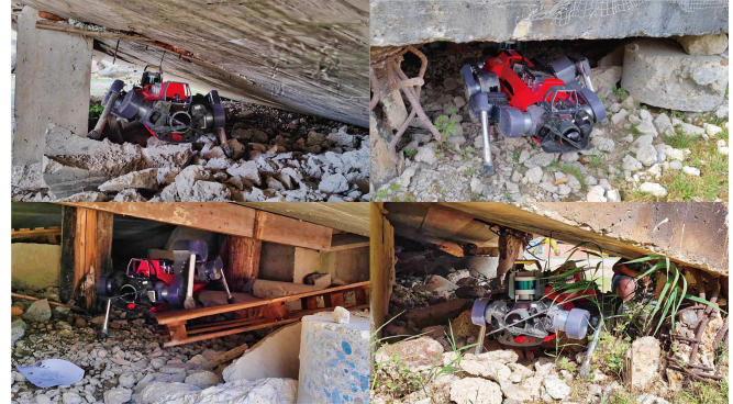
Fig. 1. Real-world experiment: Successful confined space traversal by the quadruped robot including a simulated collapsed building environment. The terrain consists of loose gravel or unstable steps, while the overhead structures have tilted configurations with narrow openings. The robot could adapt its posture to traverse these challenging conditions.
