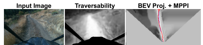
Fig. 6: Example of the projected costs and MPPI results. The blue trajectory is the expert demonstration, and the red trajectory is a result of successive application of MPPI-optimized control inputs.
