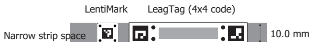
Fig. 11. Maximum sized LentiMark and LeagTag in a narrow space like a flat space in front of convenience store shelves.
