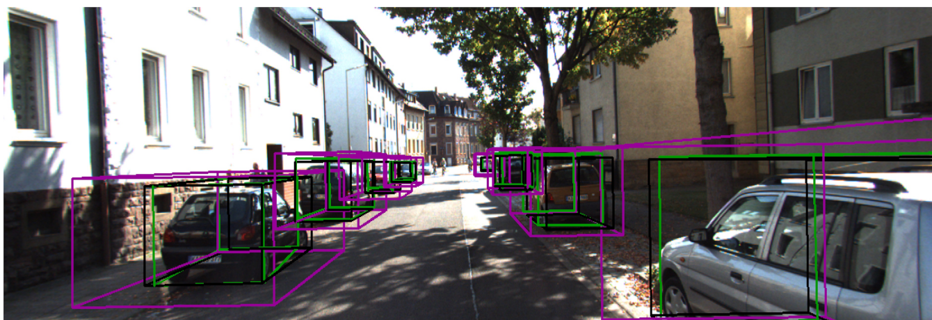
Fig. 4: Uncertainty in 3D Bounding Box Regression: Ground truth (black), predicted (green), and uncertainty (purple) 3D bounding boxes are visualized in a sample KITTI image of 8 cars with various occlusion and truncation status. As described in Section III-C, the uncertainty boxes represent a combination of upper- and lower-bound conditional quantiles obtained via conformal inference.
