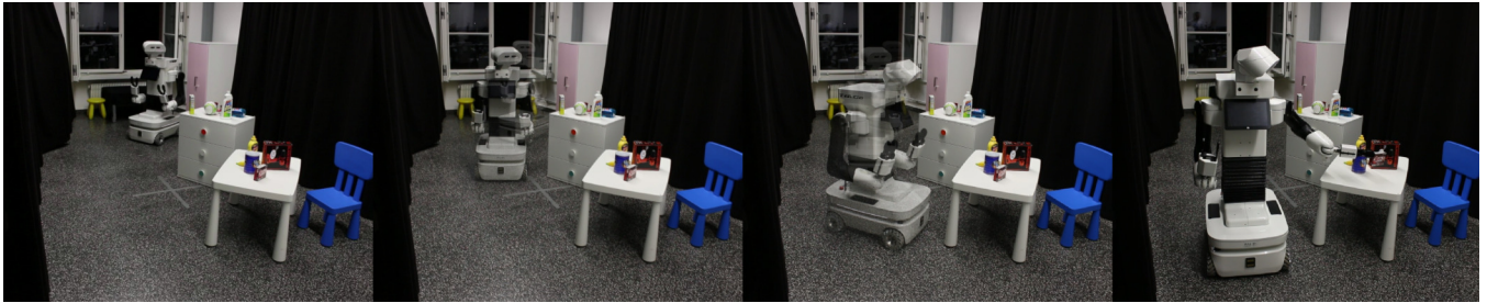
Fig. 1: Real-world execution of our active perception and grasping pipeline. The mobile manipulator robot, equipped with a head-mounted camera, efficiently explores the scene to detect grasps on the target object and effectively performs the grasp by evaluating its executability. Video demonstrations are provided in the supplementary video and the project website: sites.google.com/view/actpermoma .
