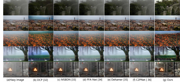
Fig. 2. Qualitative verification on the Fattal dataset [37] using state-of-the-art single image dehazing methods. Our method shows the best dehazing performance, with vibrant colors, balanced contrast, well-exposedness, and higher overall image quality.
