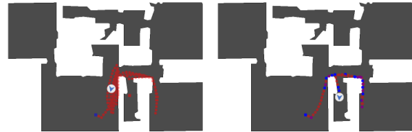
(b) The robot attempts to explore the larger rooms autonomously, it does not find the smaller room containing the goal without human intervention.
