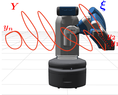
Fig. 4: The ‘Fetch.Arm - hello’ problem visualized. The sweeping motion of the robots arm is generated by overlaying the first 20 configurations from a trajectory \xi returned by CppFlow. The red cursive ‘hello’ is the target path, denoted Y . The target path Y is composed of n target poses y_1, \dots, y_n a hyperparameter set here to 175) [8]. IKFlow models are trained by fitting a Conditional Normalizing Flow model to a dataset of ground truth IK solutions. To bias the model away from self collisions, the IK solutions in the dataset are all non self colliding. IKFlow does not consider obstacles in the environment. The training procedure is covered in detail in prior work [8], [9]. IKFlow generates IK solutions as a function of a latent vector z and a target cartesian pose y , in batch on the GPU. IKFlow models empirically exhibit a desirable property: small changes to either the latent vector or target pose result in small changes to returned IK solutions. We use IKFlow as the generative-IK model because of this smoothness property and its low inference time and high accuracy.
