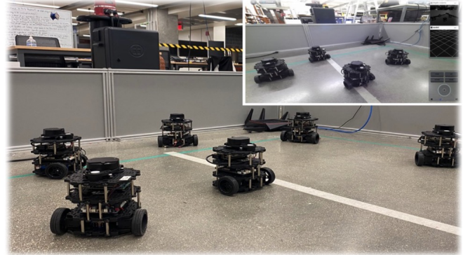
Fig. 1: This figure shows DOS ® deploy a collision-free navigation algorithm to a swarm of robots. (Turtlebot Burger). The right-top figure is the Operating page where viewing from the coach robot (Pyrobot). User can manually move the robot by the joystick the page provides.
