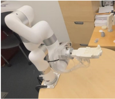
Fig. 13. 3D printed hand attached to the robotic arm.
