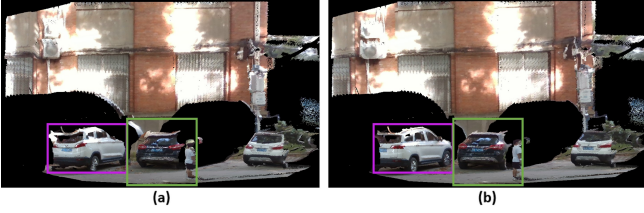
Fig. 9. Point cloud reprojection result of (a) coarse calibration and (b) fine calibration. The details of the car and pedestrian in the boxes are improved a lot after the fine calibration.
