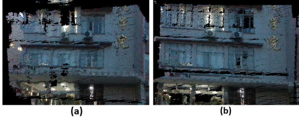
Fig. 14. The calibration result of our Velodyne VLP-16 LiDAR devices: (a) coarse calibration (b) fine calibration.
