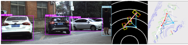
Fig. 13. The coarse calibration process using our Velodyne VLP-16 LiDAR devices.
