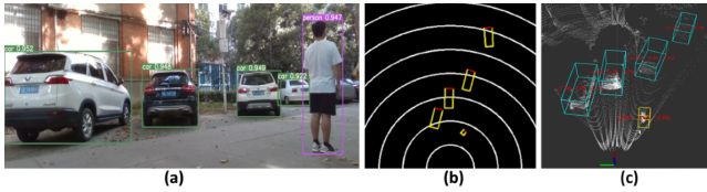
Fig. 3. (a) 2D Object detection result. (b) BEV result from monocular 3D object detection. (c) 3D object detection result in point cloud.
