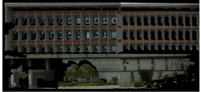
Fig. 1. Point cloud accumulated by a Livox Avia LiDAR. It is colored using an image and extrinsic parameters generated from the proposed method. The color detail of the point cloud has been restored correctly.
