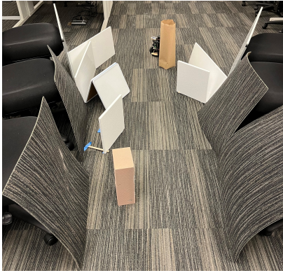
Fig. 8. The TurtleBot must move from one end of the cluttered hallway to the other without colliding with any of the obstacles.
