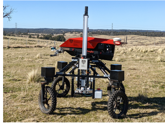
Fig. 1. The ACFR’s Swagbot autonomously collecting and analyzing soil samples.
