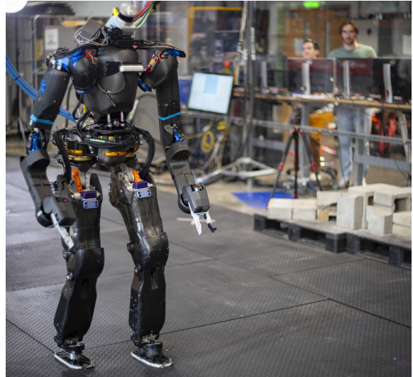
Fig. 1: Our humanoid robot, Nadia, during forward walking hardware tests of the Quickster walking controller.
