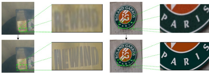
Fig. 3. Illustration of the effectiveness of the Super-Resolution unit for noise removal on underwater (First case) and natural (second case) scenes.
