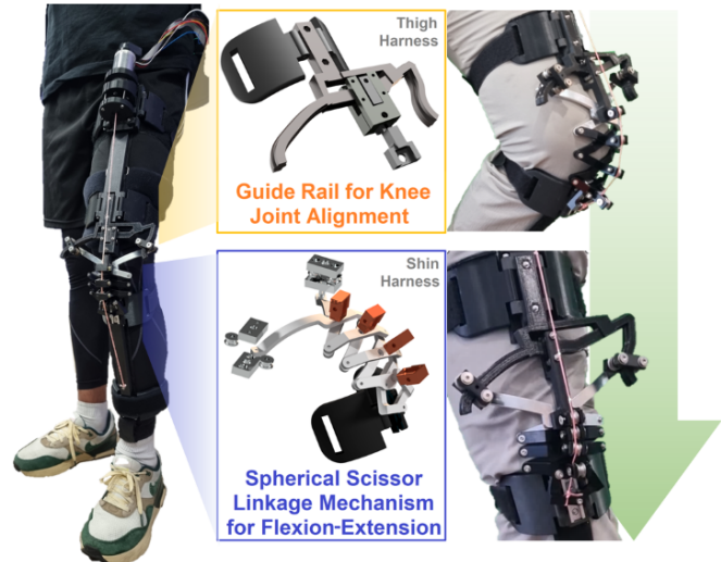
Fig. 1: Lower-limb exoskeleton with the proposed knee-joint mechanism to reduce joint misalignment. A Spherical Scissor Linkage Mechanism is used in the shin harness for knee flexion and extension, as shown by the green arrow. A customized, guiding rail is used at the thigh harness to constrain the shin harness's motion, recreating the shin's natural trajectory.
