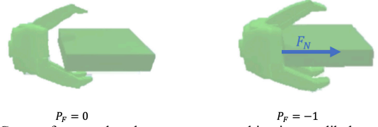
Fig 3. Contact force pushes the target away, making it more likely to miss the grip.
