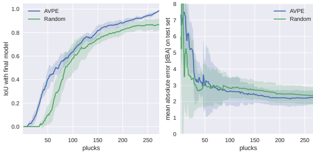
Fig. 7. (left) IoU of valid action space volumes \Phi_s^{0.75} after each new pluck and the final valid volume. Volumes were estimated through Monte Carlo integration. (right) Mean absolute error of \mathcal{D} on test set over number of recorded plucks. Both cases compare AVPE and a hypothetical random baseline.
