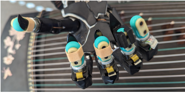
Fig. 2. Close-up view of the Shadow Hand with SynTouch BioTac sensors (turquoise), prepared with different plectrum mounts for Guzheng playing. From thumb to little finger: The thumb is taped with a specially curved Chinese thumb plectrum; two fingers with a regular Chinese plectrum taped to the fingertips as in human playing, experimental 3D-printed plectrum held in place with a thimble fitted to the finger, little finger without a plectrum, as traditional in Guzheng playing.
