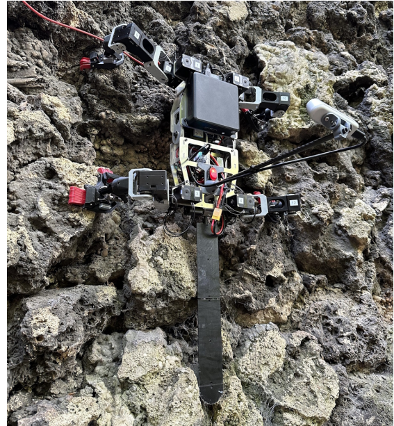
Fig. 1: The LORIS robot uses passive microspine grippers and directed inward grasping to ascend the side of a tufa stone bridge.
