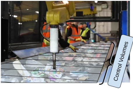
Fig. 3: Control volumes overlaid on conveyor belt serving a team of human and robot sorters
