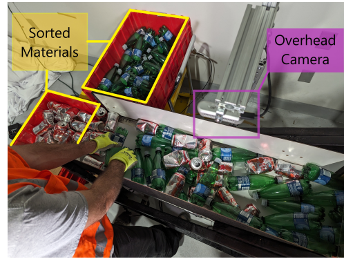
Fig. 6: Physical conveyor belt experimental setup showing the RealSense D435 overhead camera, human sorter and the sorted materials
