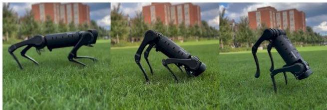
Fig. 6: Transition from quadrupedal walking to bipedal walking.
