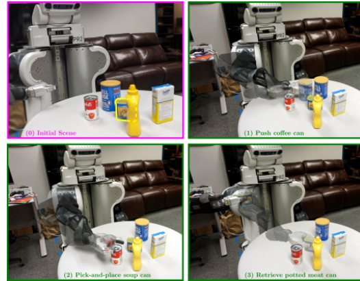
Fig. 7. A real-world MAMO problem being solved by the PR2 using I-M4M-PnP. The potted meat can is the OoI (outlined in yellow), all other objects are movable.
