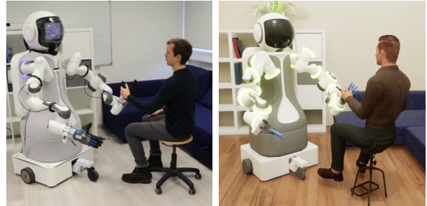
Fig. 1: An exemplary physical interaction scenario showcasing the humanoid robot GARMi and a human user. By synchronizing both the robot and human joint locations from the physical twin PT (left), physical interactions occurring in the real-world can be precisely mapped to the digital twin DT (right).
