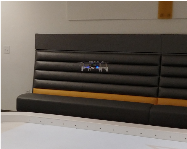
Fig. 4: A hardware demonstration of a Crazyflie nano quadcopter following a circular trajectory using our model predictive controller on ROS 2.
